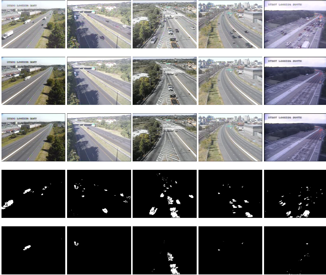
Figure 1. The foreground detection and background estimation performance of the proposed method. The first row shows some video frames from the NJDOT traffic videos with a spacial resolution of 352 \times 240 . The second row shows the background estimated using the GMM method. The third row shows the background estimated using our novel GFM guided background modeling method. The fourth row shows the foreground mask detected by our method. The fifth row shows the stopped foreground objects detected by our method.
