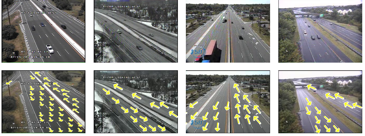
Fig. 4: Extracting a matrix of motion flow vectors using GMM method with optical flow vectors as input. First row contains sample frames of traffic videos. Second row represents the corresponding flow model matrix obtained from the GMM method.
