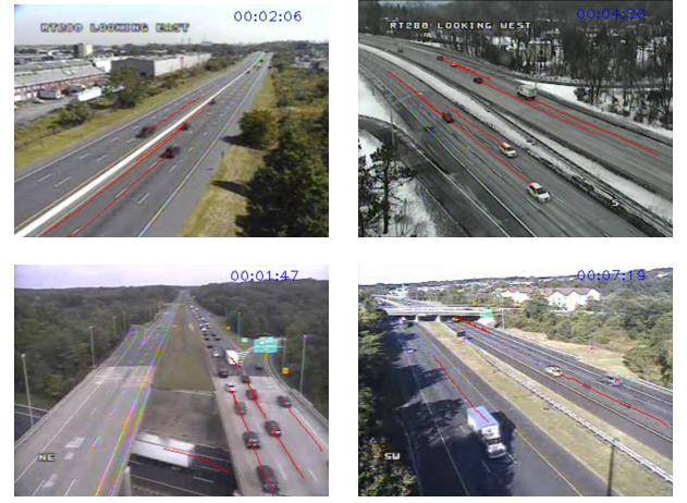
Fig. 3. The moving trajectories detected by our new MOT method. The red lines indicate the moving trajectories of the vehicles in two seconds.
